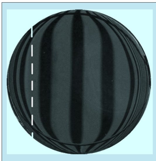
Figure 3. In a convex surface a cross-section intersects the reflections of multiple rafters.
