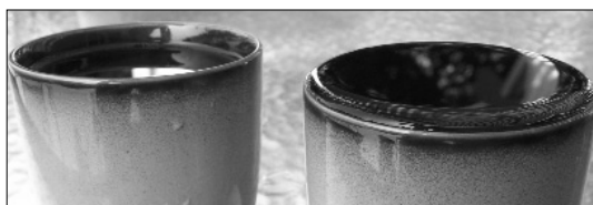
Figure 2. (Left.) A partially full cup of tea has a concave surface. (Right.) However, in an overfull cup of tea the surface is convex.
