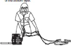
4. Use the plastic strap (attached to the bottom rung) to wrap and secure both layers of rungs. This will minimize the chance of the ladder becoming tangled when you remove it from the box in an emergency.
