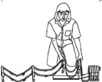
Stack a second layer of rungs 12 thru 22 on top of the bottom layer.
