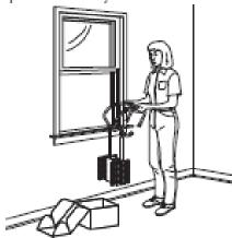
Place the sill hooks firmly over the windowsill and pull the release strap to deploy the ladder.
